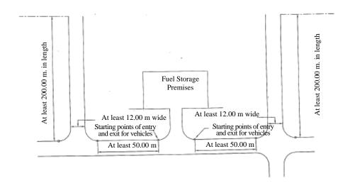
Showing steepness of the slope where entry and exit for vehicles are not permitted to be located in fuel storage premises.
