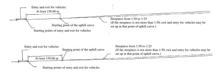
Showing the starting or ending points of a bridge ramp where its steepness is not more than 1:50
