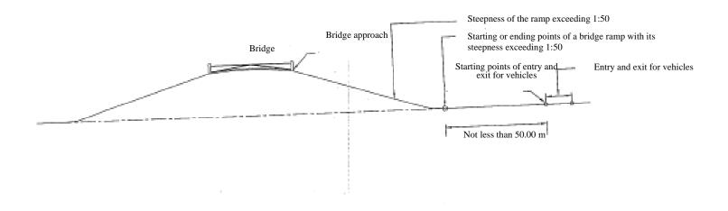
Showing the starting or ending points of a bridge ramp where its steepness is not more than 1:50
