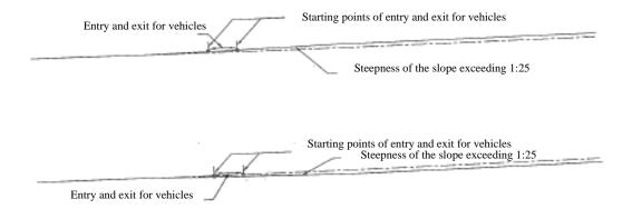
Showing the distance between starting points of entry and exit for vehicles in fuel storage premises to the starting point of a curve of an access way with a gradient on Either side from 1:50 to 1:25.
