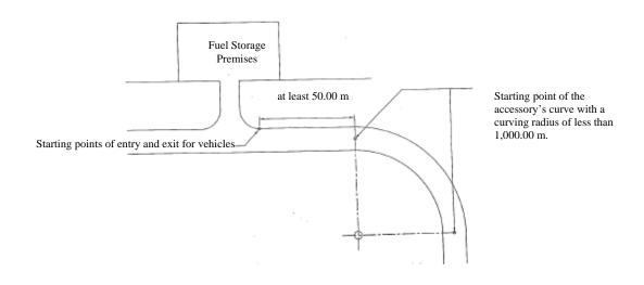
Showing the distance between starting points of entry and exit for vehicles in fuel storage premises and the starting point of a junction's curve.
