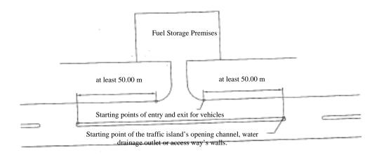
Showing the distance between starting pints of entry and exit for vehicles in fuel storage premises and starting point of the access way's curve with a curving radius of less than 1,000.00 m.
