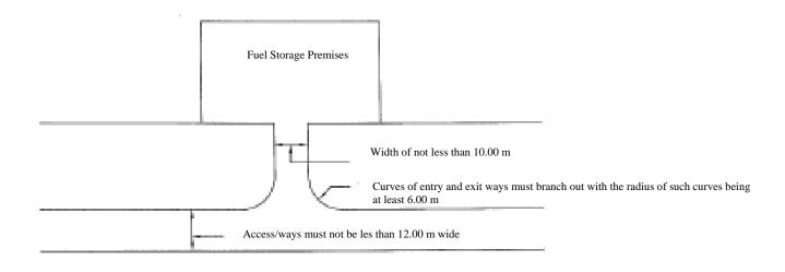
Showing the distance between starting points of entry and exit for vehicles in fuel storage premises and those of the traffic island's opening channel, water drainage outlet or access way's walls.
